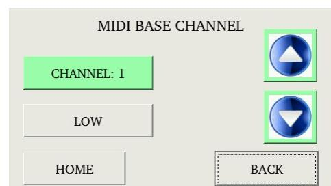
To change the MIDI Base Channel, touch the CHANNEL button to highlight it, then use the UP and DOWN buttons to change the MIDI channel value.
